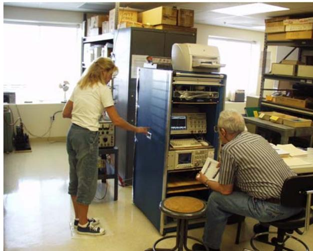
Figure 3. Photo of real HBM test configuration with human “volunteer” touching the current sensor
