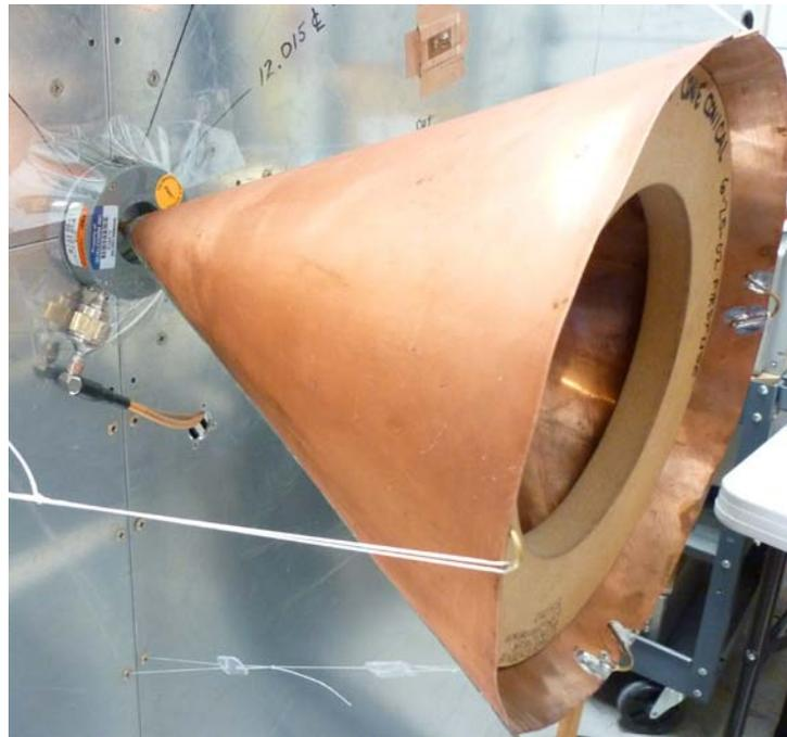
Figure 1. The 12 inch long, 100 ohm, copper conical radiator with Fischer probe
