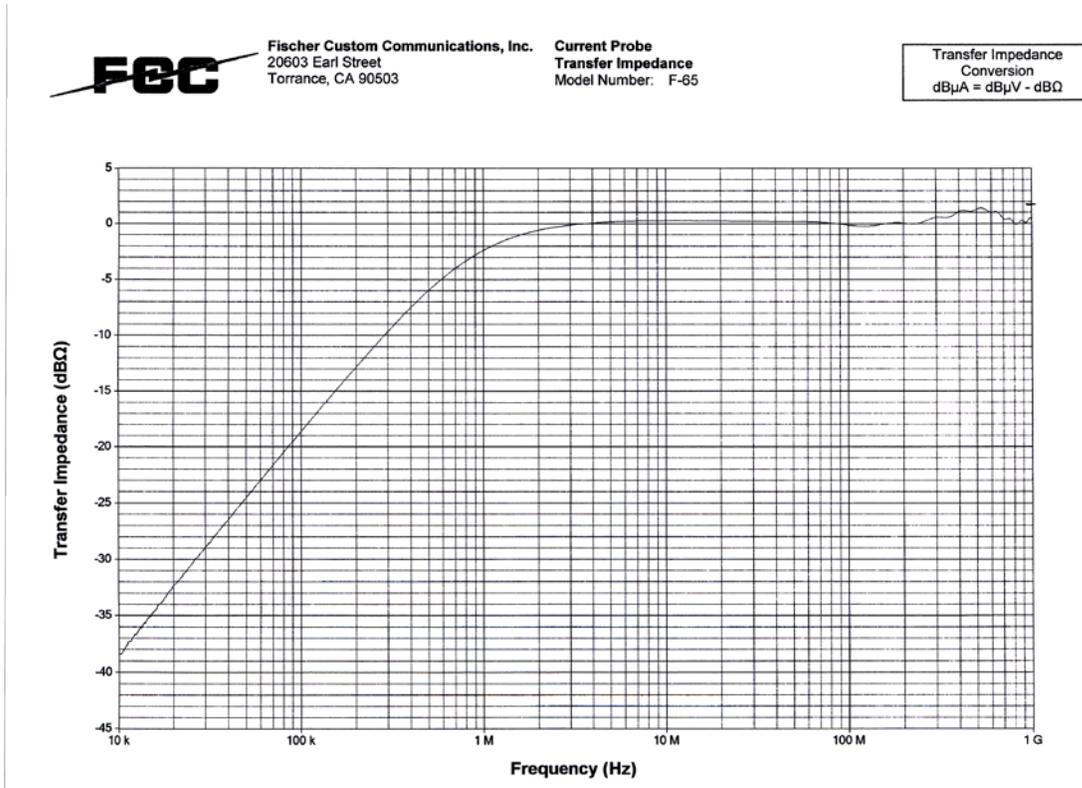
Figure 5. Fischer F-65 Current probe response in the frequency domain
