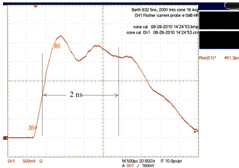
Figure 2. Fischer Current probe pulse response with 12 inch conical radiator
