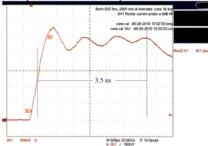
Figure 4. Fischer Current Probe pulse response extended out to 3.5 ns
