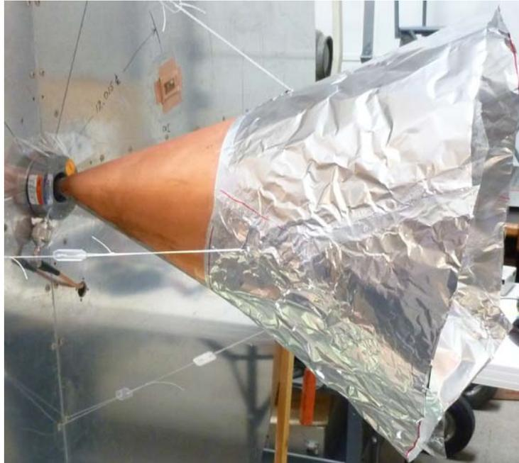
Figure 3. Extended length 100 ohm conical radiator with Fischer probe
