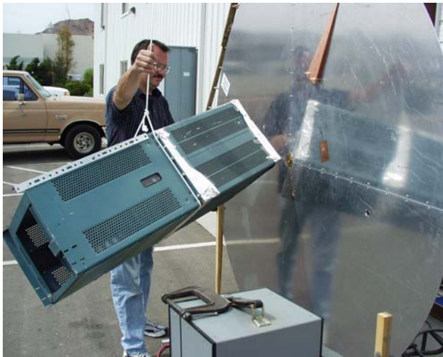
Figure 5. Photo of real MM test configuration (using 18”x 40”x 14” enclosed frame).
