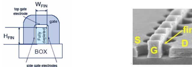
Figure 17: Cross-section of an advanced FinFET.
