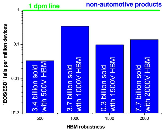
Figure 13: EOS/ESD fails of non-automotive ICs returned to IC supplier versus the achieved HBM qualification level. A total number of nearly 15 Billion parts is considered.
