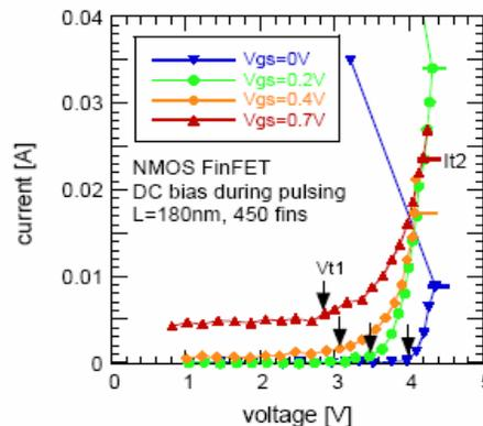
Figure 18: I<sub>ds</sub>-V<sub>ds</sub> curves for varying gate bias with trigger voltages (V<sub>t1</sub>) and failure currents (I<sub>t2</sub>) shown for a FinFET device structure [5].
