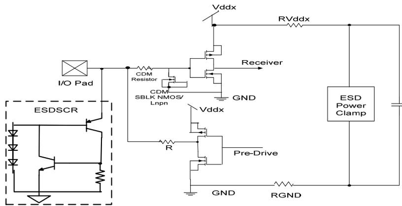
Figure 24: Diode String Triggered SCR (DTSR) with RC-triggered Rail Clamp ESD Protection Strategy
