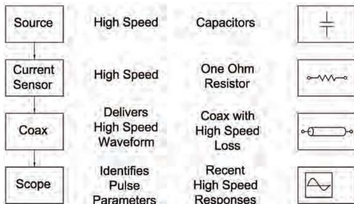
Figure 1. CDM Measurement Chain
