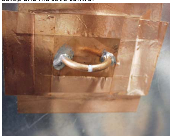
0.190" gap H loop through 36" Semflex low loss coax, + 10" QMI coax, with 0dB SMA atten. 12.015" from target (current probe) center to center line of sensor
