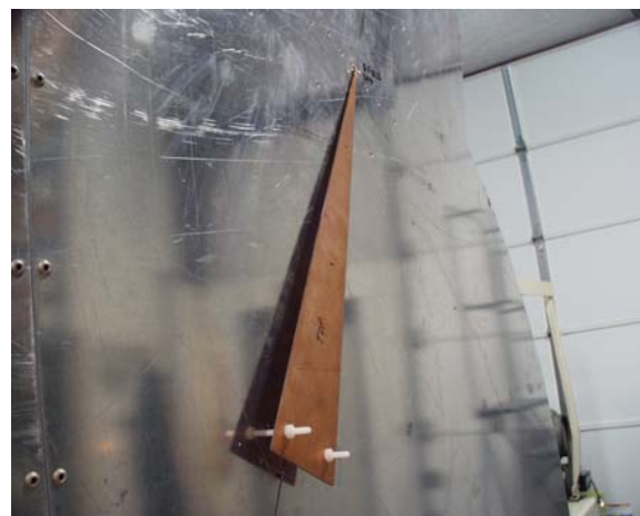
E Field 14" TEM horn w/ 0.65" aperture 16.25" from center of target, +36" Semflex low loss coax, w/ BE 142-20 SN 42 10.022VR Pulse atten.
