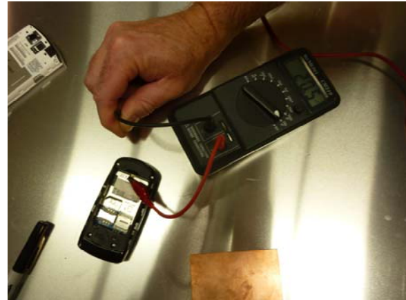
Small phone to gnd capacitance measured 21pF
