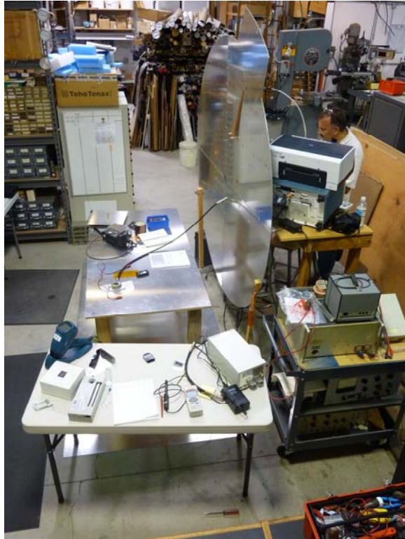
Test setup showing 2M ground plane, IEC Test bench with floor ground plane.
