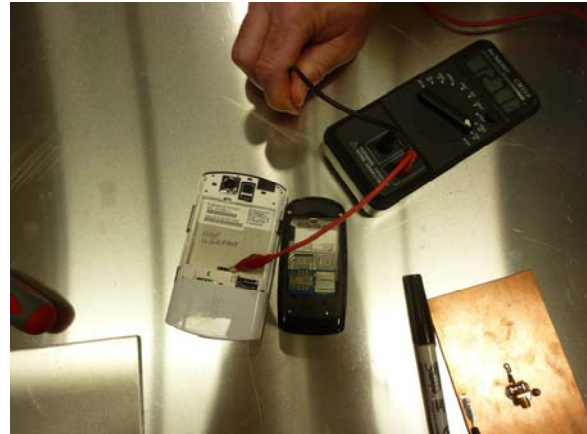
Large phone to gnd capacitance measured 132pF
