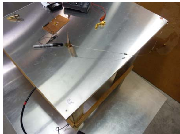
Capacitance measured table top to ground plane 18.9pF (w/ground resistors disconnected).
