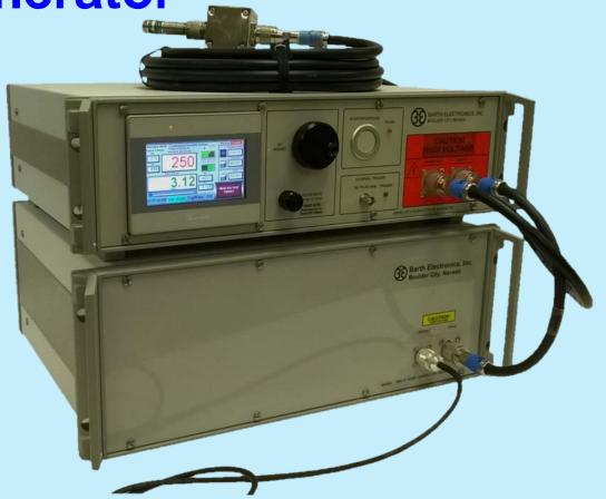
Barth Common Mode Transient Generator was developed for Common Mode Transient (CMTI) characterization testing
