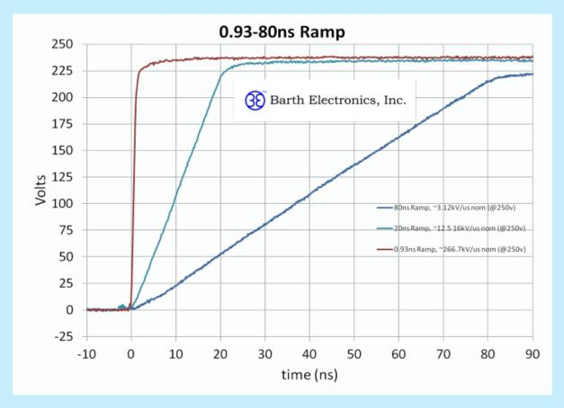
Samples of 0.93ns, 20ns, and 80ns ramp output showing leading edge of pulse into a matched 50 ohm load
