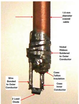
Figure 2. 1N4148 diode mounted on coax
