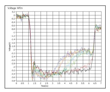
1. The lowest voltage data point is the black trace where it is relatively constant throughout the length of the five (5) nanosecond test pulse.
