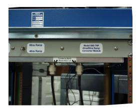
Unit connects to the external rise time spoiler connections on the 4002-TLP to provide both 40 and 80ns rise time linear ramp function to the TLP test system.
