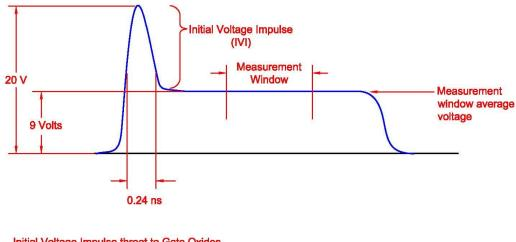
Initial Voltage Impulse threat to Gate Oxides Caused by delay in semiconductor conductivity
