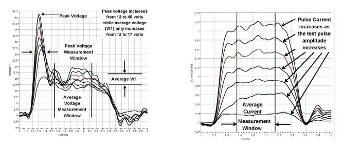
The voltage and current waveforms shown above are of a snapback device. The Voltage waveforms show the Vt1 voltage increasing from 12V to 17V while the peak voltage added threat to the Gate Oxide increases from 12 to 40 Volts. Measurements on wafer; and of packaged devices provides a completely new understanding of CDM circuit operation inside the package.
