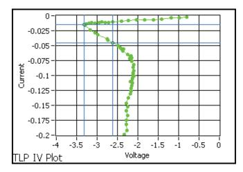
The 4012 VFTLP+ software uses two blue cursors used to select two I-V data points which includes all the data points between them. The seven (7) green DUT data points select the all the voltage and current waveforms to be displayed on two more screens for analysis of turn-on characteristics.
