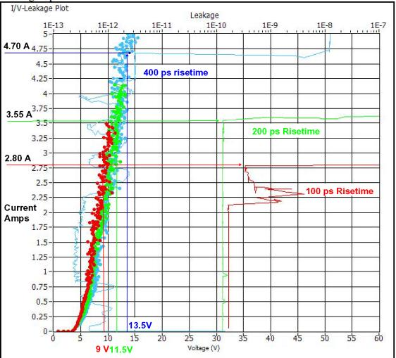
This above plot shows the ordinary I-V plot of a protection circuit which begins conduction at 4 volts and reaches 10 or 15 volts at currents where the gate oxide fails. The ordinary I-V data averaged during the measurement window at late time doesn't provide the data needed. Current, is not what damages gate oxides however; the short impulse of voltage is the real threat.
