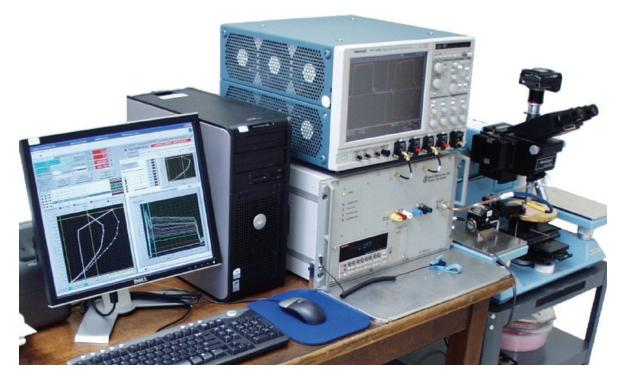
VFTLP+ now provides revolutionary improvement in understanding CDM effects inside the package. This test is now available to help you analyze your CDM circuit design. Very Fast test pulse and Measurements simulate the very fast CDM event. Understand the very fast operation of your voltage clamping circuits for the first time.
