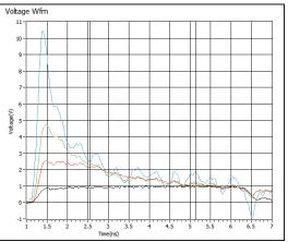
Figure 3. Voltage waveforms of 1N4448 diode There is no current created when the 1 volt test pulse is applied to the diode, as shown in the black trace. The slow increase in current is obvious in the next test pulse (red) as the current requires almost 4 nanoseconds to reach its constant amplitude.
