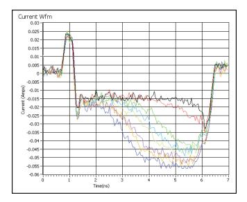
1. Again the lowest test pulse amplitude is the black trace which is relatively constant throughout the length of the five (5) nanosecond test pulse.
