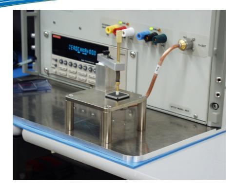
The Universal Test Fixture is designed to be used with the Model 4012 VFTLP+ Test System for packaged part testing. A packaged DUT is placed dead-bug style on the ground plane, with the pin to be pulsed contacting the pin protruding from the base. The return pin is connected to the base through a special clamp to the baseplate. The vertical plunger and additional clamps insure the DUT is held in position.
