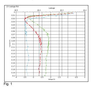
The blue plot shows how the device turns on at 1 ns pulse width. The pulse is so short that the circuit doesn't have sufficient time to fully conduct into snap-back mode. its An approximate measure of the negative resistance at the slight snap-back conditions indicate that it would be about -0.60 ohms. This short pulse test shows that the circuit cannot get into its higher conduction made to cause the
