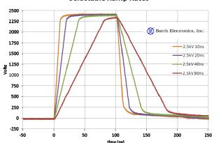
Barth Electronics latest invention turns step functions into ramp functions
