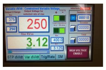
"VAR" variable dV/dt mode shown features a continuously variable dV/dt selectable by the user.
