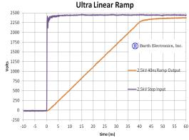
This ramp generator design is very scalable allowing fast to slow ramp rates in 2:1 steps, and outputs from very low voltages, to very High voltages, positive and negative polarity, limited only by the connector and cable capabilities.
