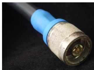
**463-NMMP** One (1) N Male connector assembled on each end of RG214/U coax; Maximum voltage specification is 3kV DC.
