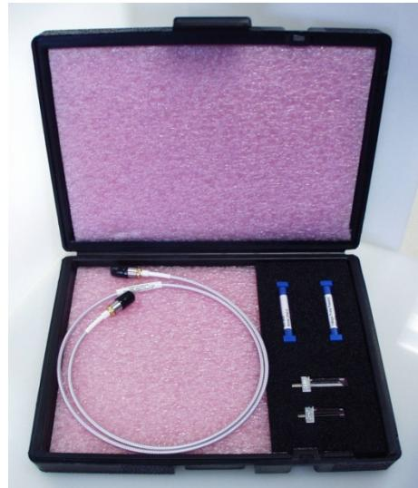
Note: The probe ratings are for use with the supplied 36" long low loss cable. Use of longer or higher loss cable will degrade the risetime of the measured pulse.
